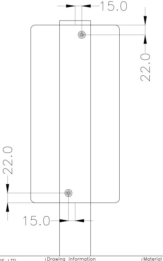
CRITICAL HOLE DRILLINGS OFF CENTRE TO AVOID SCREWS CLASHING
