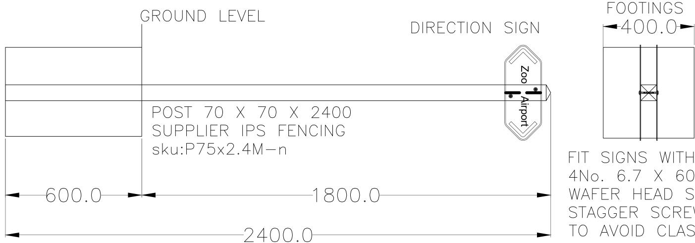
FIT SIGNS WITH 4No. 6.7 X 60 WAFER HEAD SCREW STAGGER SCREWS TO AVOID CLASH
