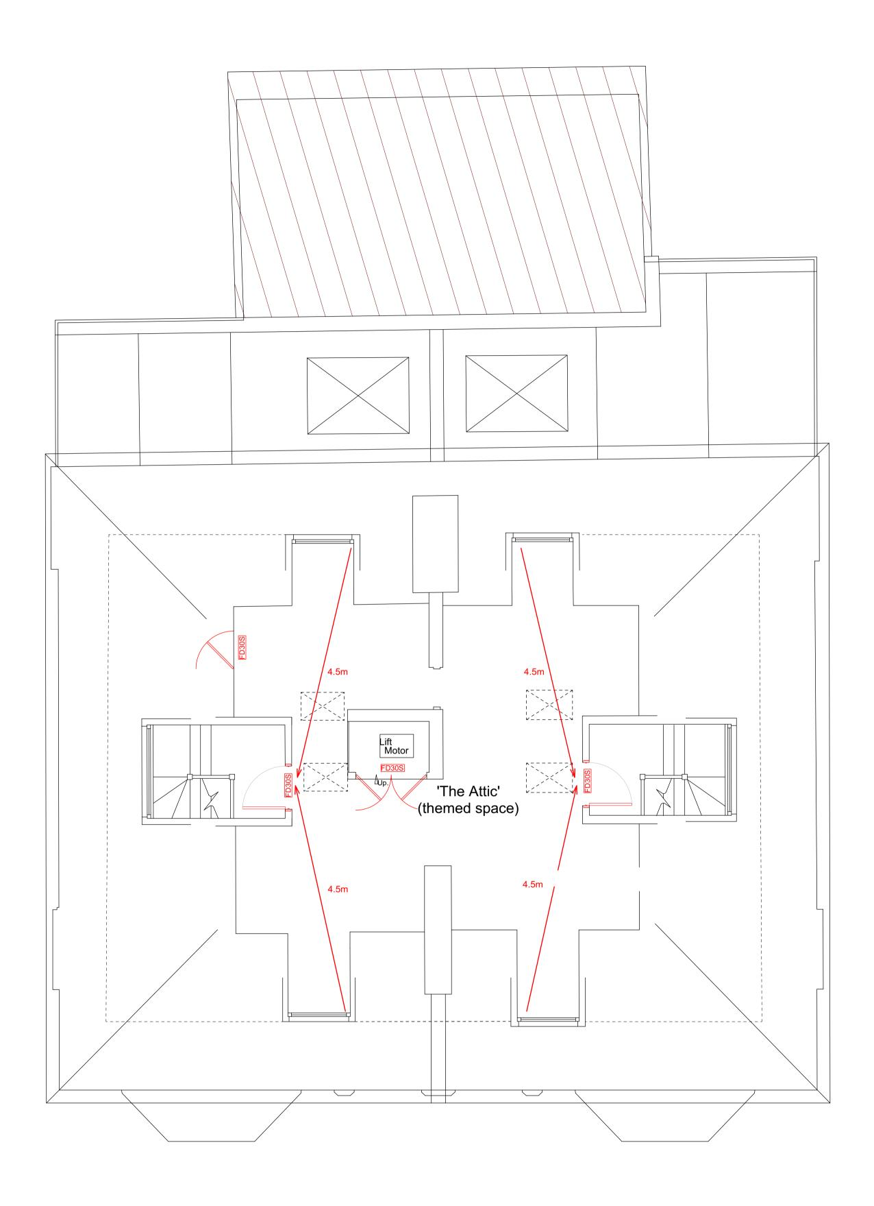
Notes Fire Safety Existing F.E Final Exit <sup>1m</sup> Escape Distances 750 Clear Width 30 min fire rated TBC (see ironmongery schedule) S.C Self closer FD30S Self closer and smoke seals EXIT Emergency exit sign
