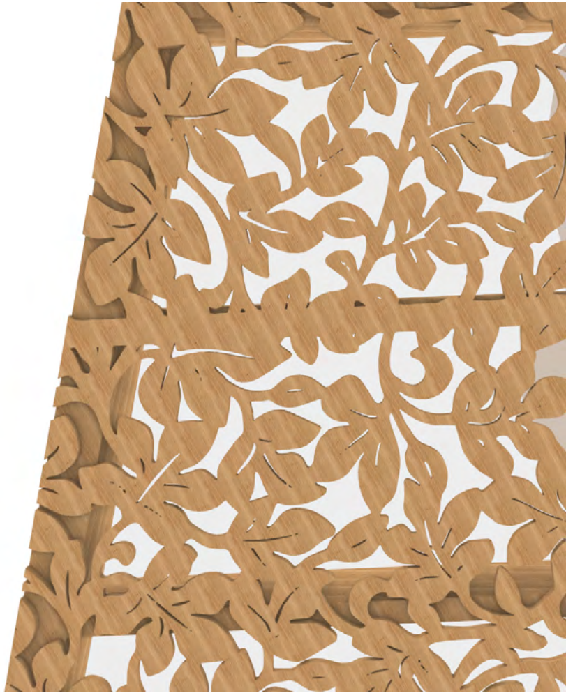
Laser cut douglas fir plywood pattern to main canopy roof
