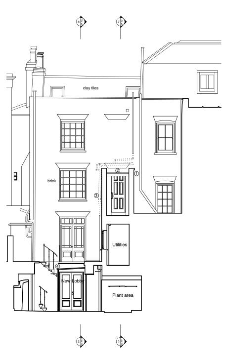
① - new glass skylight obscured behind new parapet, parapet raised in brick to match existing in brick, bond and pointing capped with cast stone coping
