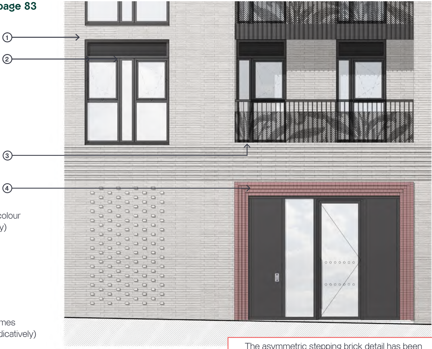
1 Lower Block Ground Floor Shop Fronts - Bay Study Elevation 1:25
