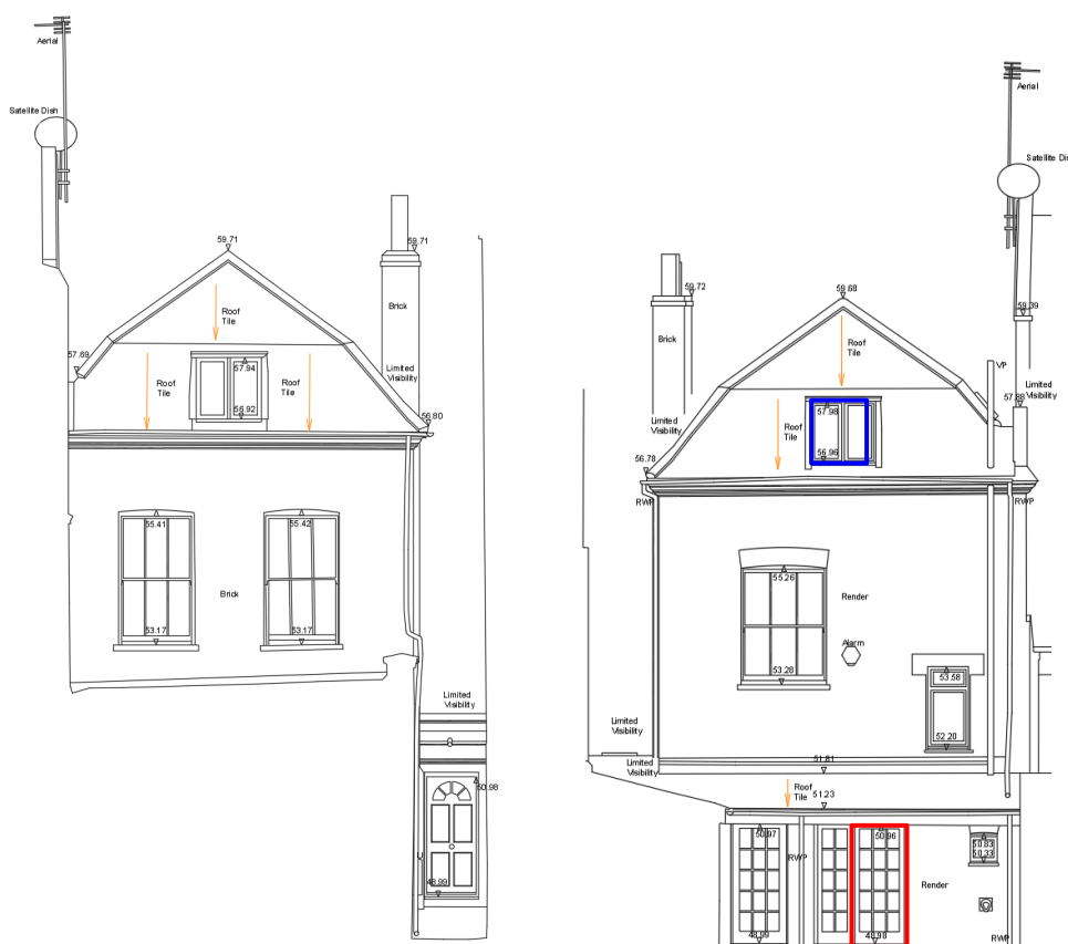
Figure 2: Window opening details – Front and rear elevation
