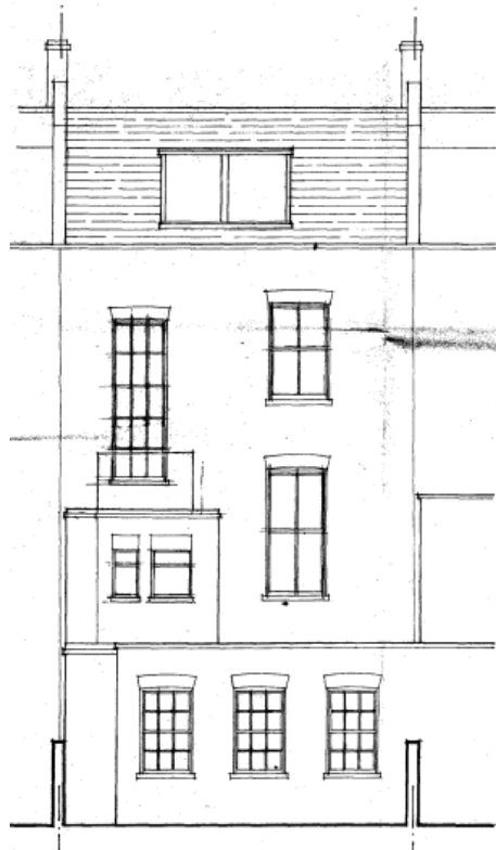
Figure 12 1988 permission (ref: 8870177) showing existing rear elevation with later two over two sashes and dormer windows.
