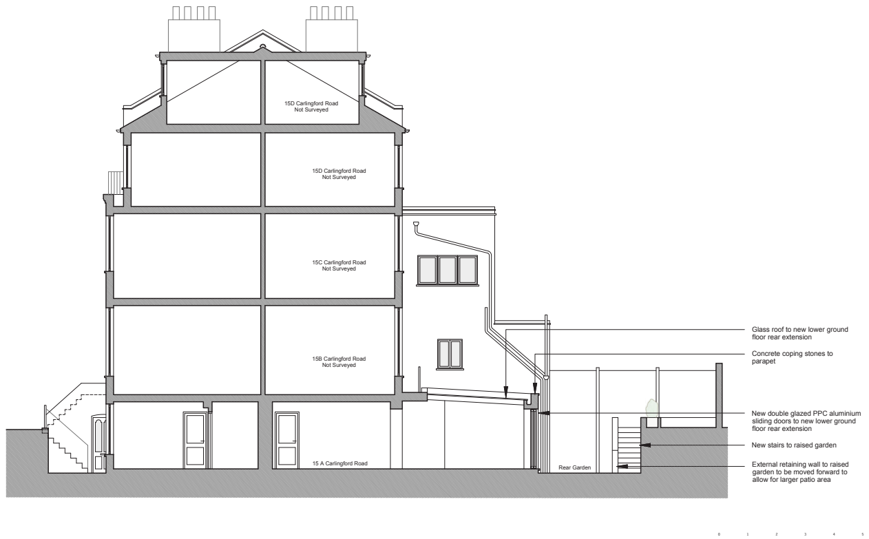
Section drawing showing the proposed new side return rear conservatory extension and patio garden steps to the Lower Ground Floor Flat.
