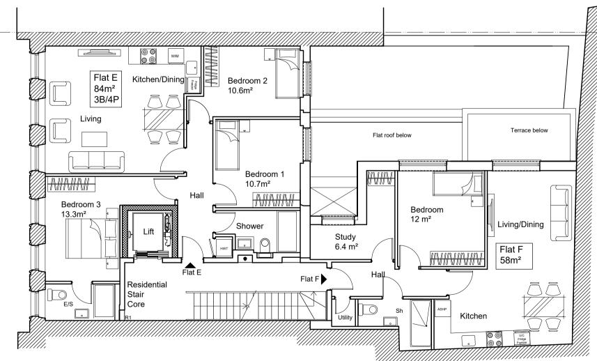
Proposed Second Floor Plan Scale 1:100
