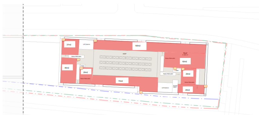
Figure 6: PBSA PV Roof Array
