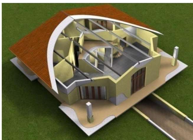
Figure 9: Cut-away of Heavyweight Structure (Thermal Mass)
