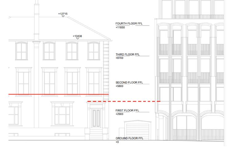
Drawing A214 - <u>All window sizes and their details are wrong</u> and need to be re-surveyed and redrawn in relationship to the proposal. Red line = approximate true height of door and lintel. Dotted line = incorrect lintel height lining up with first floor windows (the only features that line up).
