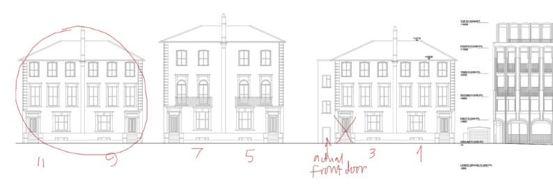
2) A second error shows No.3 with steps up to a front door: in reality the front door is in a stairwell addition built in the 1960's when the house was made into flats. The applicant's survey failed to notice this obvious fact.
