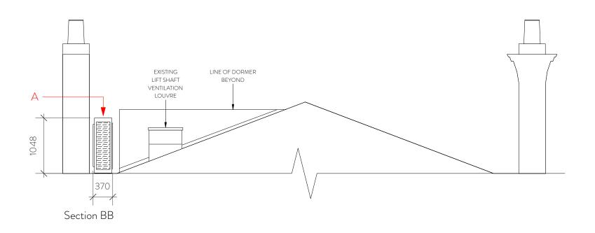
Condenser Model: MXZ-6F122VF-E1 Manufacturer: Mitsubushi Fixed on Cantilever Brackets mounted on chimney breast fixed into brick mortar joints
