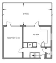
PROPOSED GROUND FLOOR PLAN SCALE 1:100 @ A3
