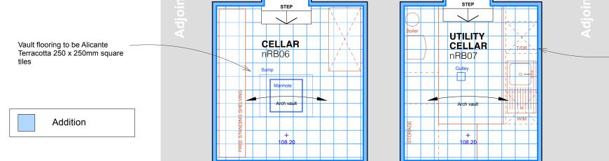
Floors and walls of Storage Cellar and Utility Cellar to receive waterproof lining (highlighted in blue). Fitout design of cupboard and storage units shown by others.
