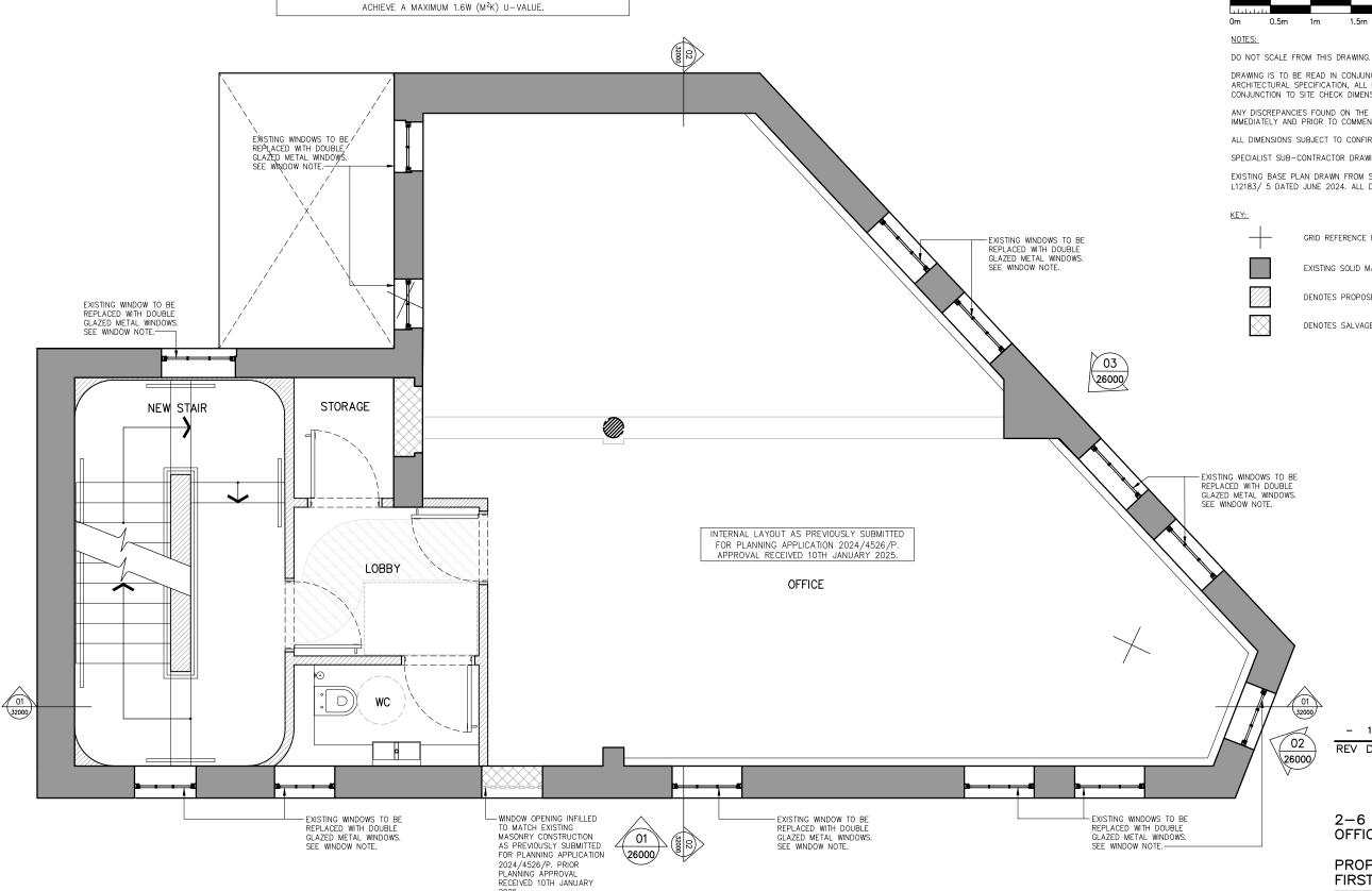
WINDOWS WHERE NOTED EXISTING SINGLE PANE CRITTAL WINDOWS TO BE REPLACED WITH DOUBLE GLAZED METAL WINDOWS WITH METAL FENESTRATION TO RESEMBLE THE
