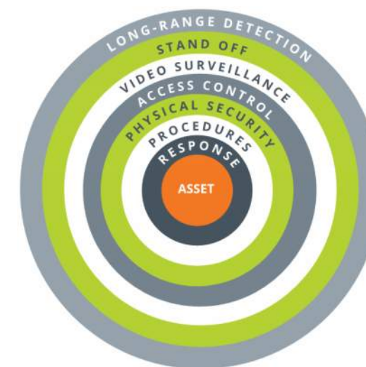
Figure 21 Layering of security measures (Toren)
