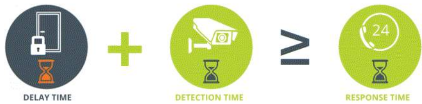
Figure 22 Time to delay and detect an intruder should be less than time to respond (Toren)
