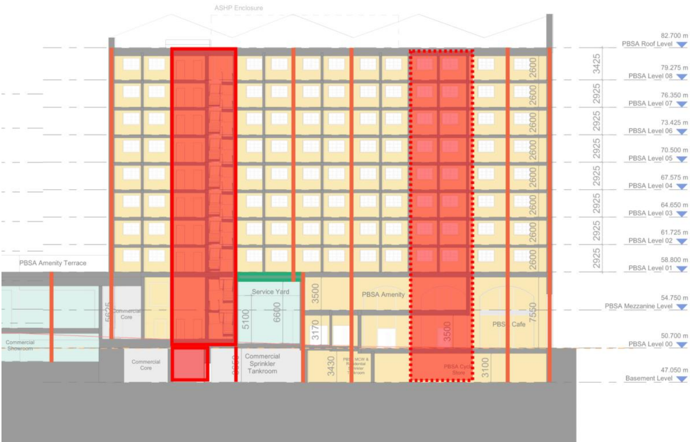
Section of PBSA block indicating lateral stability structures in red
