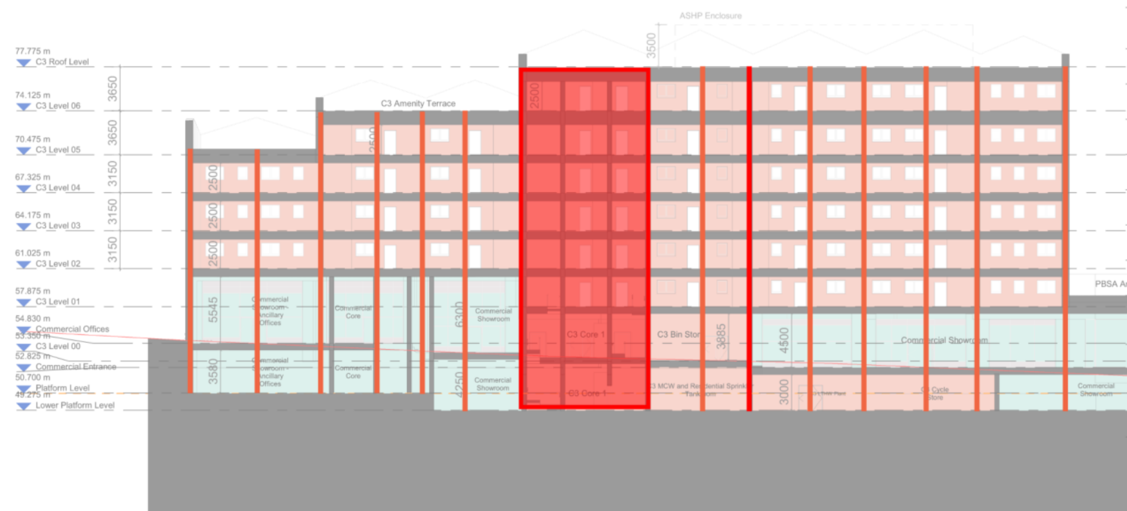
Section of residential block indicating lateral stability structures in red
