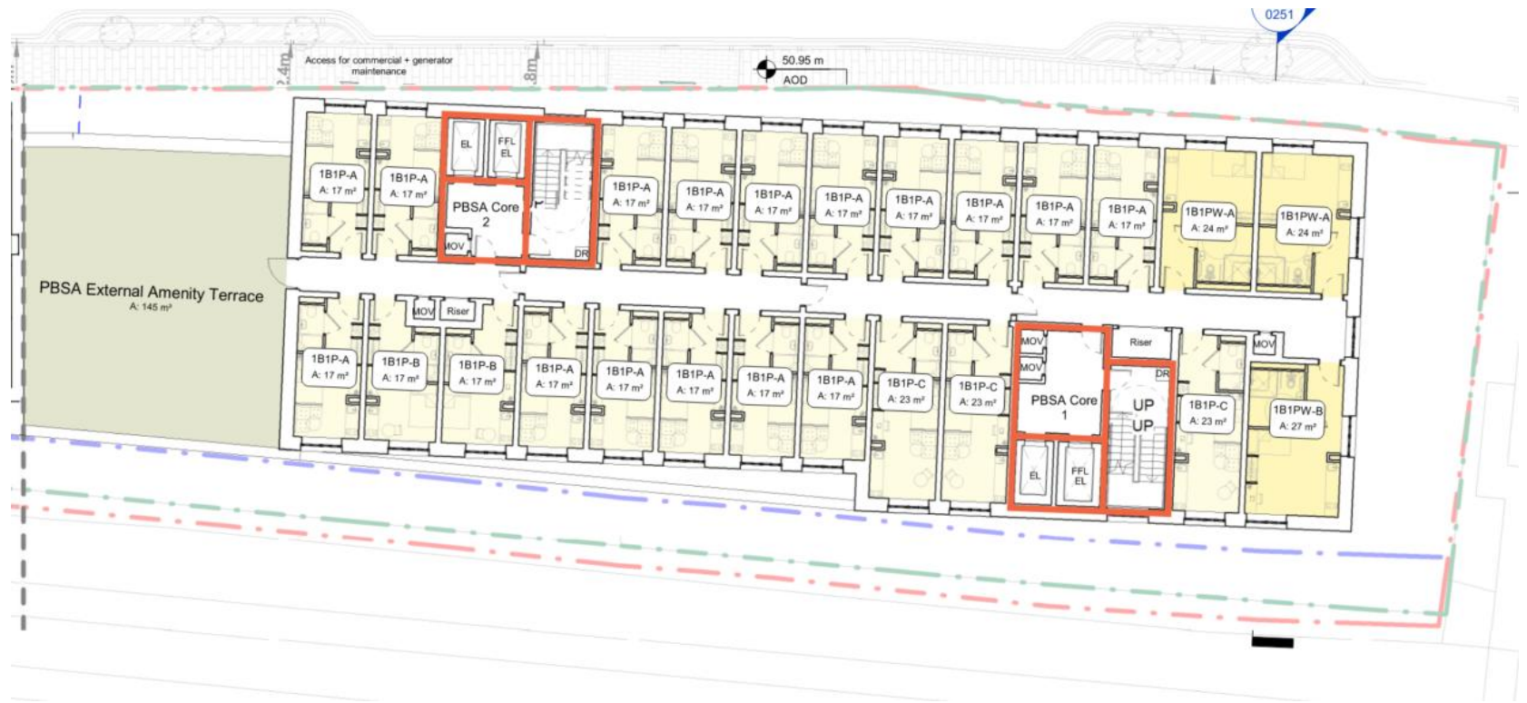
Plan on typical upper floor of PBSA block indicating lateral stability structures
