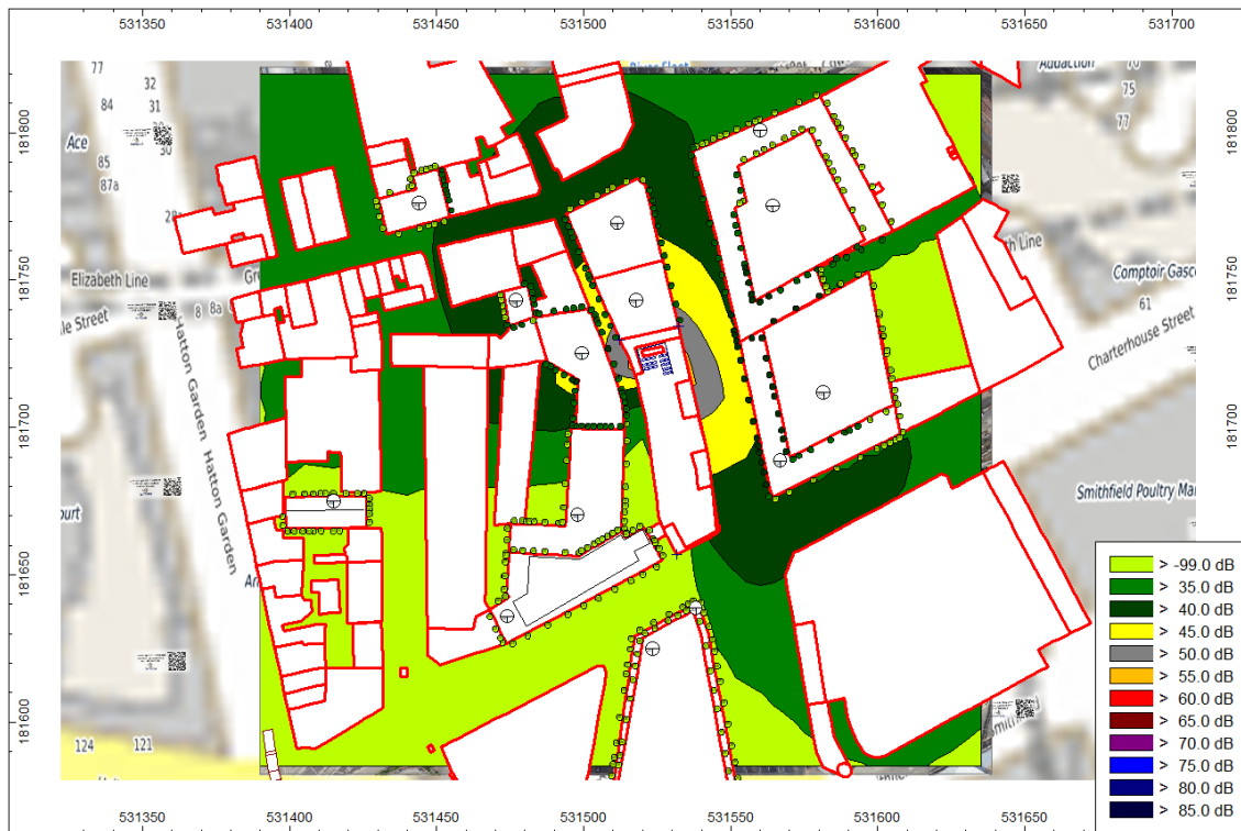
Figure 4: Specific noise level contours, dB L_{Aeq,T} , for Typical Plant. Office hours.
