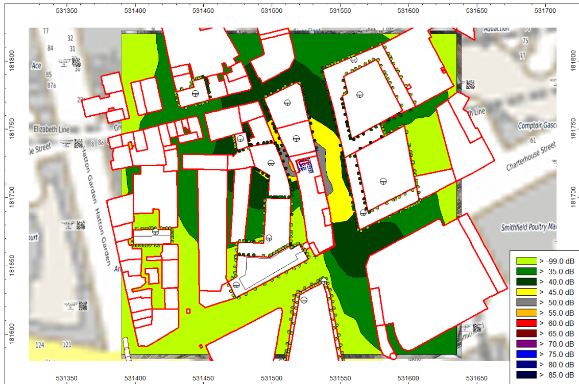
Figure 4: Specific noise level contours, dB L_{Aeq,T} , for Emergency Plant. Night-time hours.
