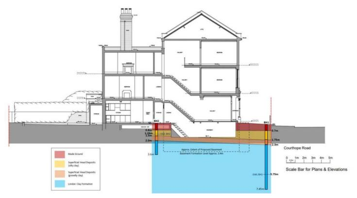
Figure 3: Ground Model (existing section from STAC Architecture Limited 'General Arrangement Elevations & Section A-A & B-B as Existing).
