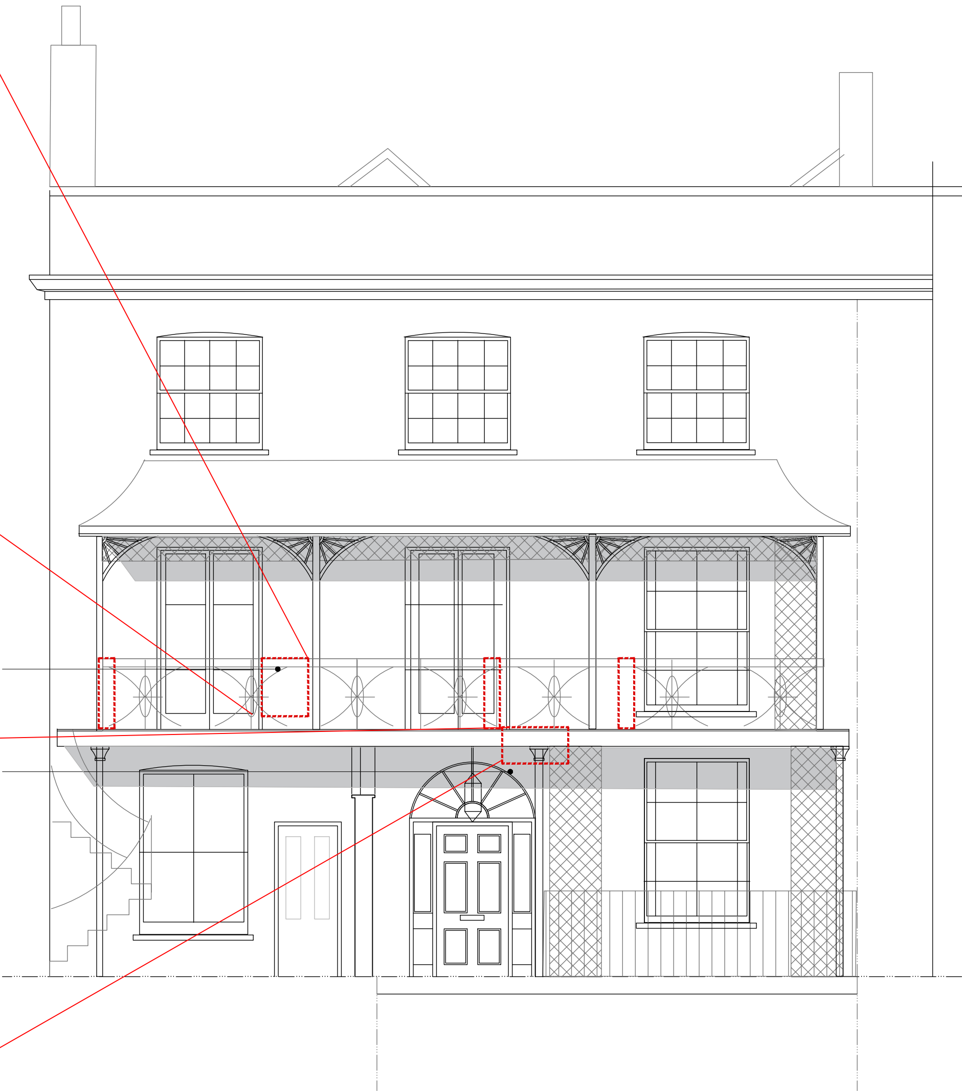
TIMBER JOISTS ROTTED AND SOME BOARDS REQUIRING REPLACEMENT TO BALCONY.
