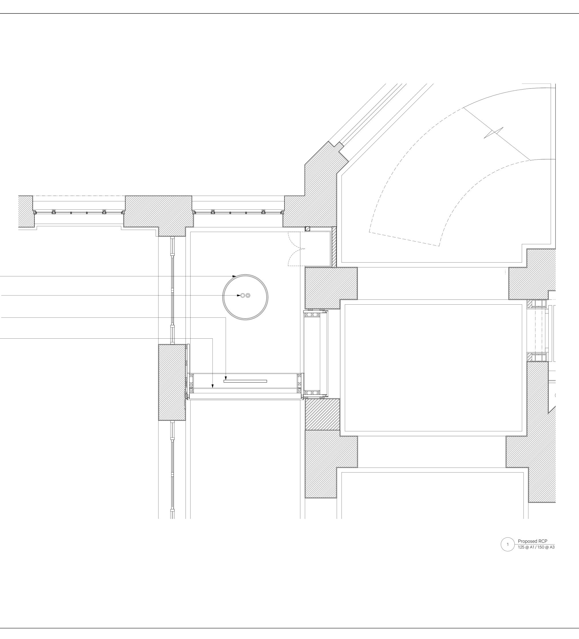
New suspended circular direct/indirect pendant luminare
