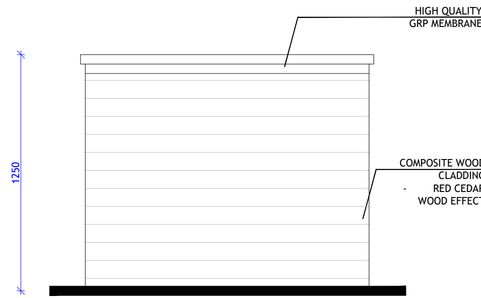
TIMBER BIN STORE - FRONT ELEVATION SCALE 1:20
