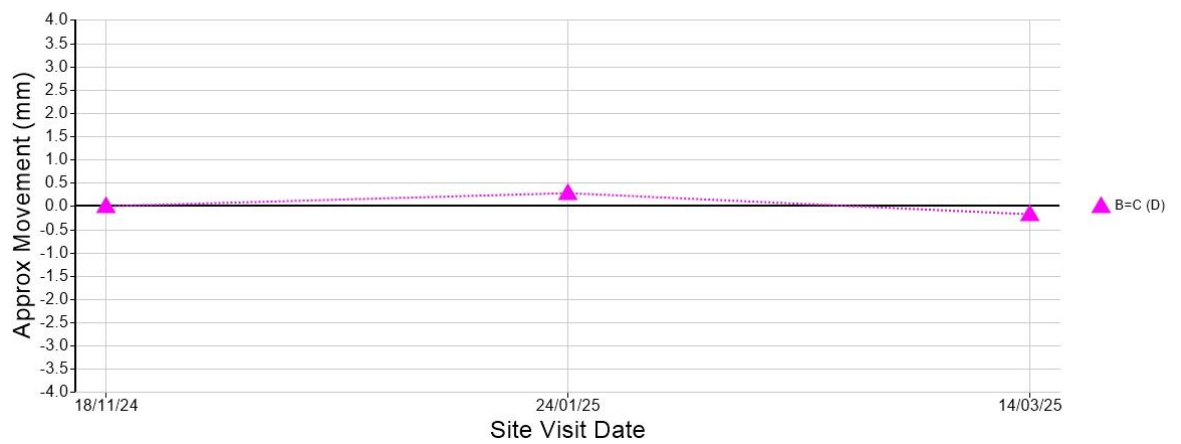
C5 - INT - right hand wall in lounge left hand side of opening to kitchen
