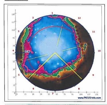
The yellow line on the tomography indicates the likely presence of internal cracks which are more defined then previously.
