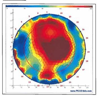
The additional red areas on the outside of the stem around sensor 7 to 10 and particularly sensors 15 to 18 indicate restrictions in sap flow likely a response to the competitive environment.
