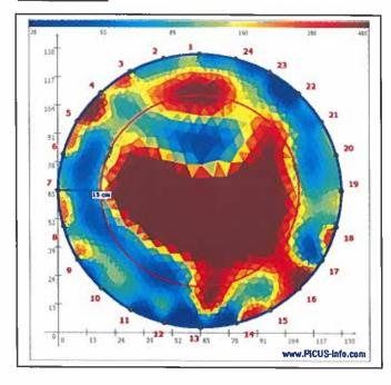
The outer stem has a higher moisture content which is assumed to be related to moisture storage during the dormant period.
