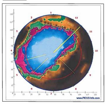
The yellow line on the tomography indicates the likely presence of internal cracks, which may have accelerated the spread of the decay fungi and may have adversely affected the tomography by increasing the time of flight for the sound signal.
