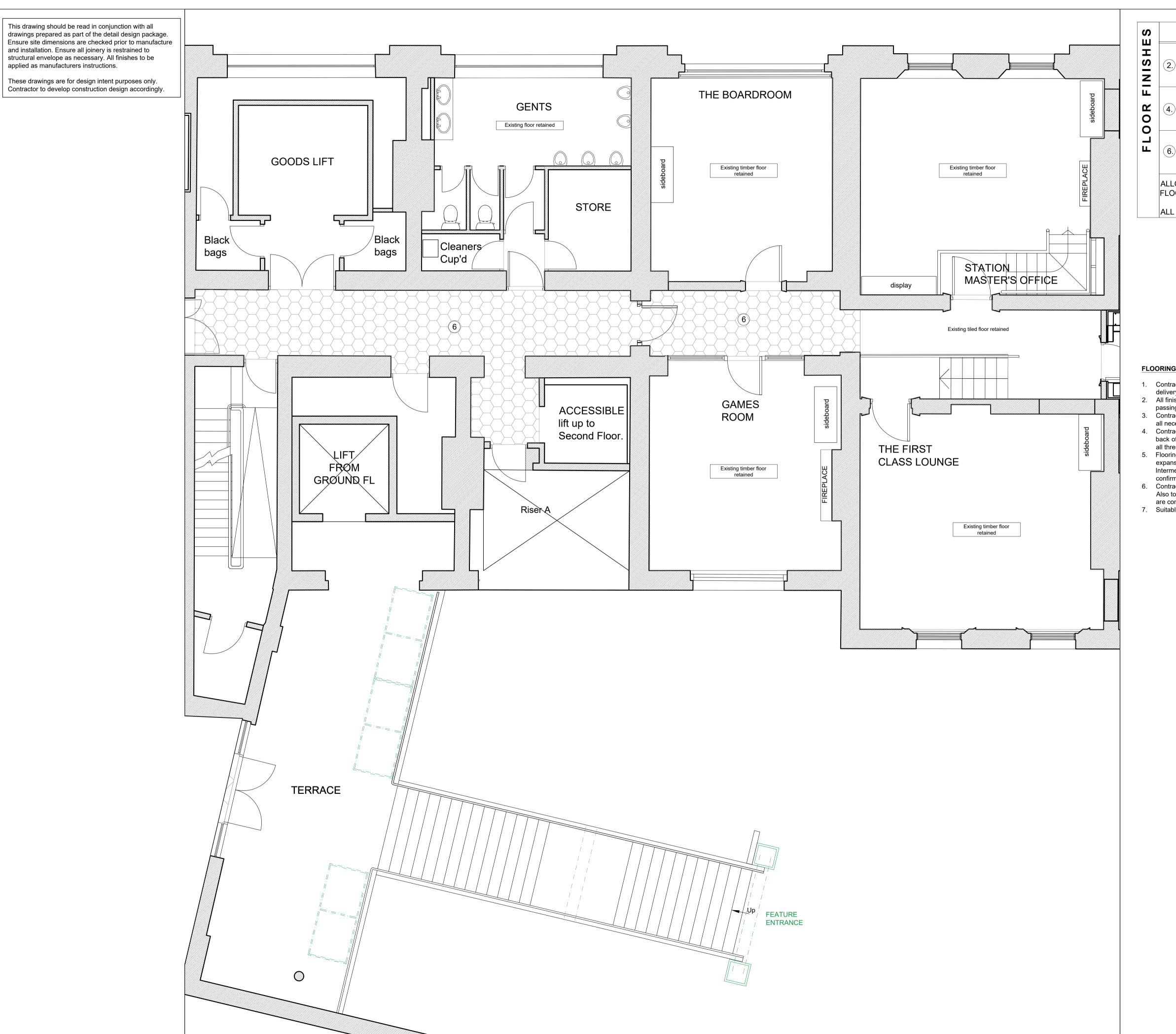
Specification Symbol Description Specialist decorative finish over | Specialist - Hana Sunny existing timber floor Safety Floor - Altro Supply and lay new Altro safety flooring with welded seams and Ref: Stronghold30 K3001 coved skirtings etc (black). Vinyl - TBC Supply and lay new sheet vinyl ALLOW FOR SILICON SEALANT AROUND ALL SANITARYWARE JUNCTIONS WITH
