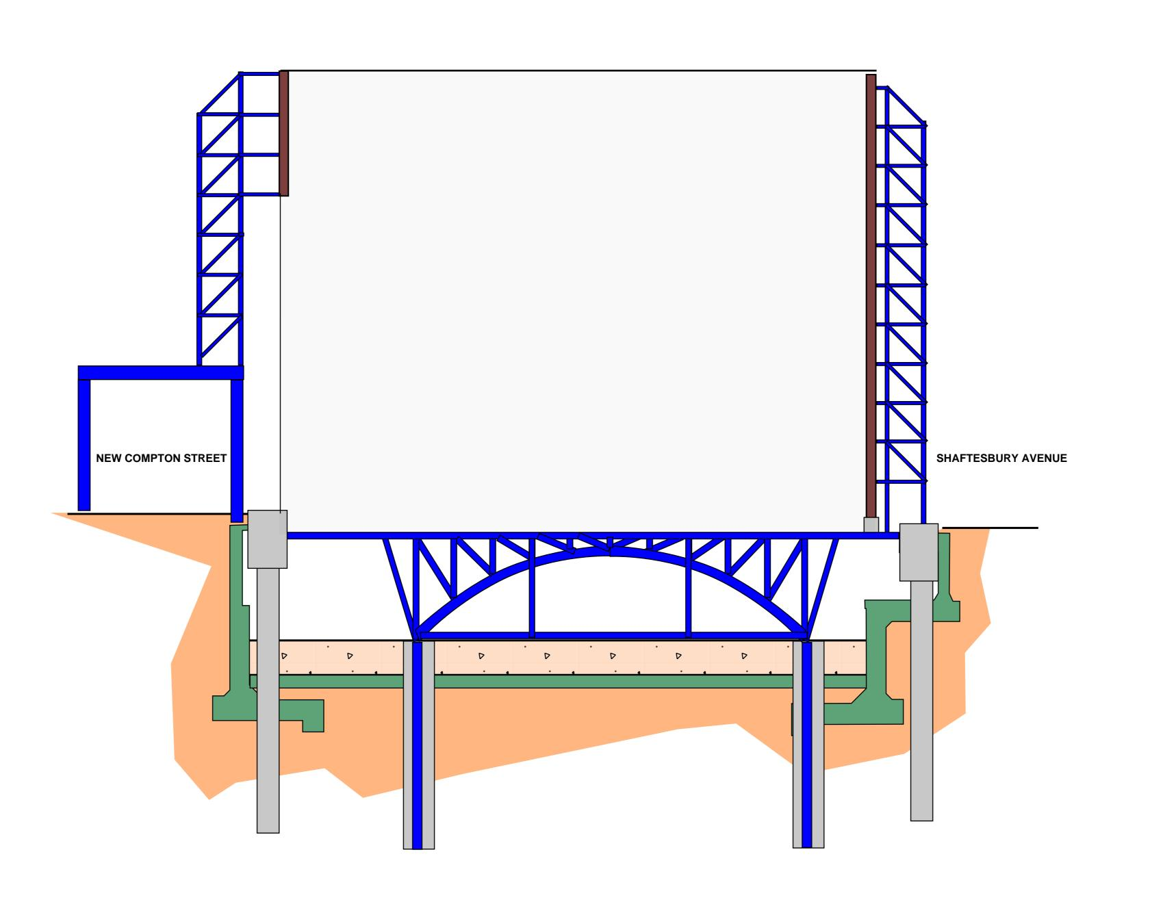
REMOVE PILING MAT DOWN TO NEW B1 MEZZ LEVEL AND INSTALL TRANSFER ARCHES.
