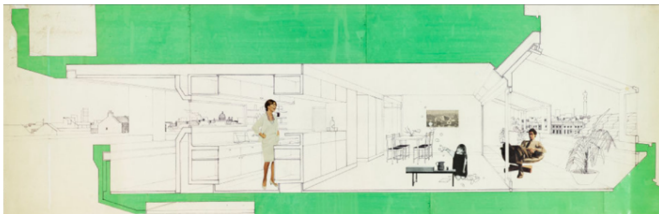
Cut-away drawing of the showing the planned interior of a flat in the Brunswick Centre before the winter gardens were reduced in size in 1966 (RIBA)
