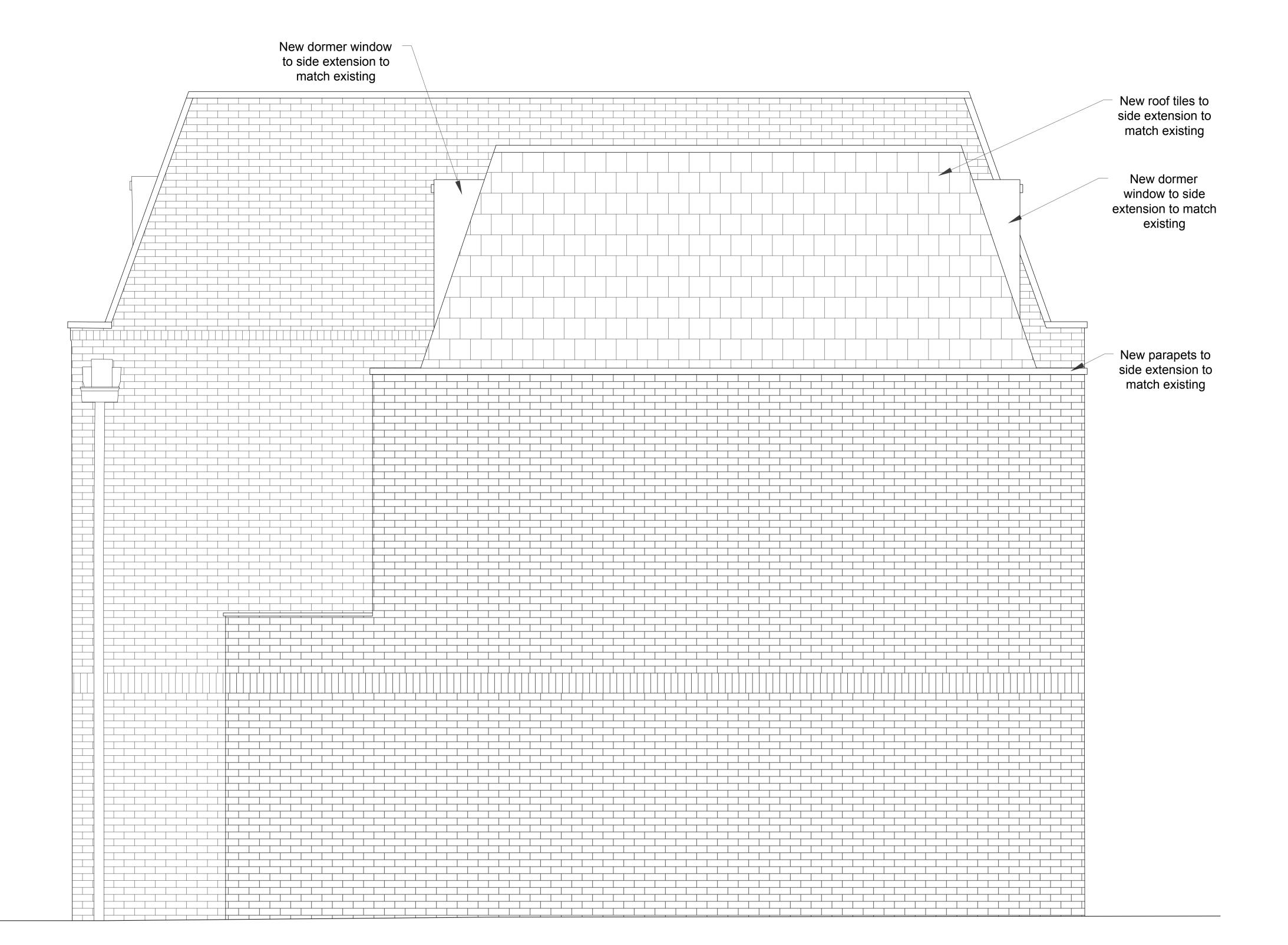
Proposed Side Elevation Scale 1:50@ A3 | 1:25 @ A1
