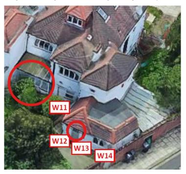
These windows are either situated alongside a projecting element or beneath an eave overhang, both of these design factors can limit sky visibility and can make windows somewhat sensitive to changes in daylight. As such, we recommend that the VSC assessment is updated and the NSC study is undertaken to these areas to ensure that the potential impact on daylight to this property as a result of the proposed development is appropriately considered.
