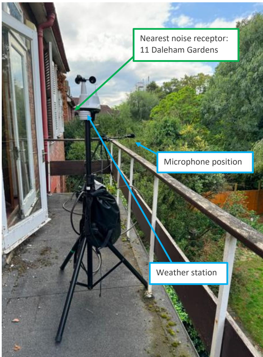
Figure 3: Sound level meter and weather station in situ in relation to nearest noise-sensitive receptor
