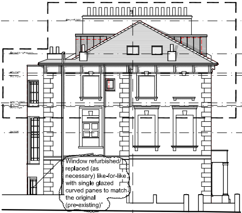
PROPOSED SIDE ELEVATION SCALE: 1:200@A3
