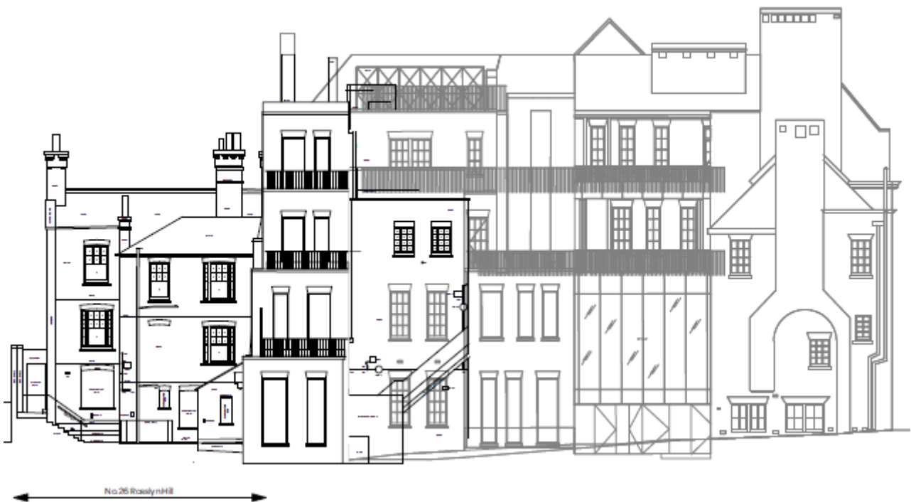
Rear elevation of consented police station scheme indicating four storey infill extension adjacent to subject site (left side)
