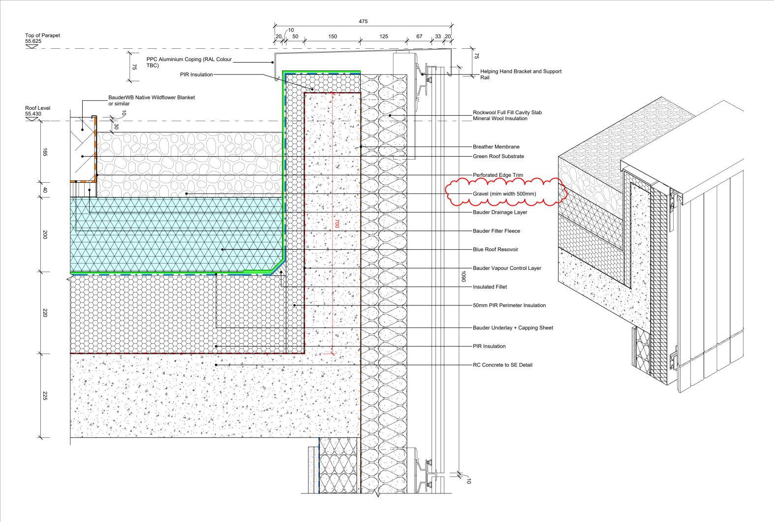
rd.18 - Top Roof Parapet 500 (gravel) —AOV/Access Hatch (Bilco or similar) -Aluminium Peel Bar (As Required) BauderWB Native Wildflower Blanket —Bauder Vapour Control Layer -Bauder Underlay + Capping Sheet Roof Level 55.430 RC Concrete to SE Detail -Bauder Filter Fleece -Green Roof Substrate -Perforated Edge Trim -Bauder Drainage Layer -50mm PIR Perimeter Insulation −Bauder Vapour Control Layer RC Concrete to SE Detail
