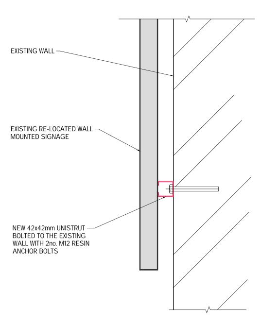
PROPOSED ENLARGED SECTION SHOWING FIXING DETAIL INTO WALL (SCALE 1:5 AT A1)
