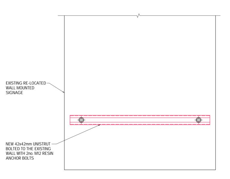
PROPOSED ENLARGED PART ELEVATION SHOWING FIXING DETAIL (SCALE 1:5 AT A1)
