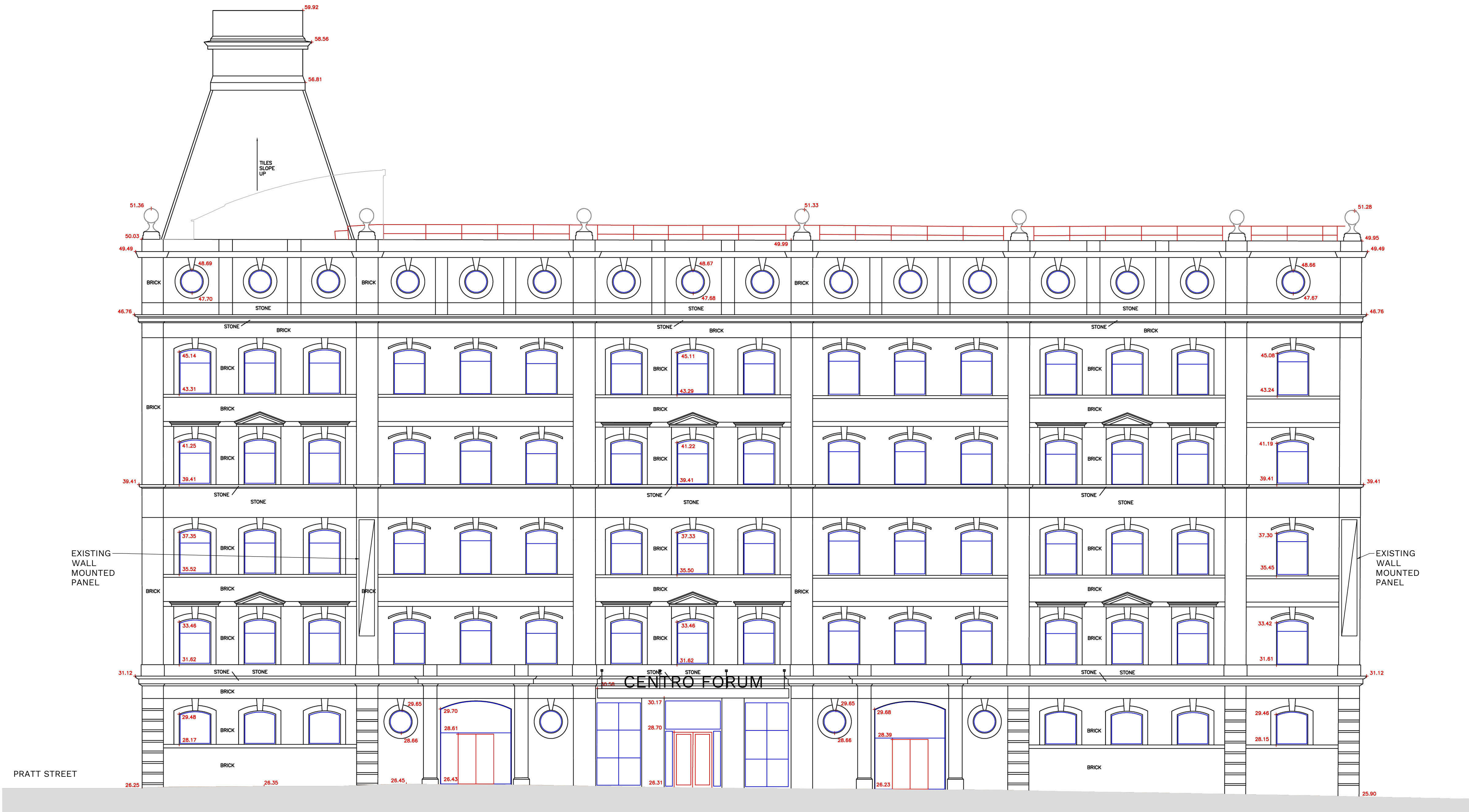
EXISTING CAMDEN STREET ELEVATION (SCALE 1:100 AT A1)
