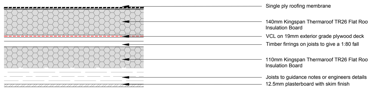
New Build Typical Hybrid Flat Roof Detail Not to Scale : Thickness/Angles as to Guidance, 1:50 and Site Dimensions by Contractor
