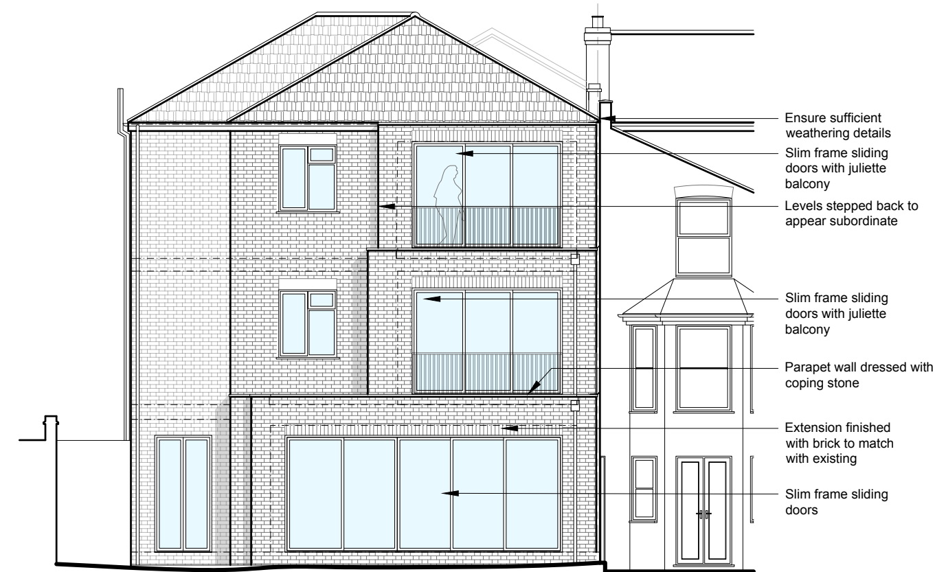
Flats - Rear Elevation As Proposed 1:100
