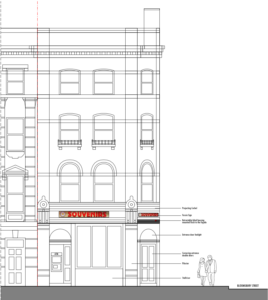
EXISTING FRONT ELEVATION - GREAT RUSSELL STREET (CANOPY IN CLOSED POSITION) Scale:1/100
