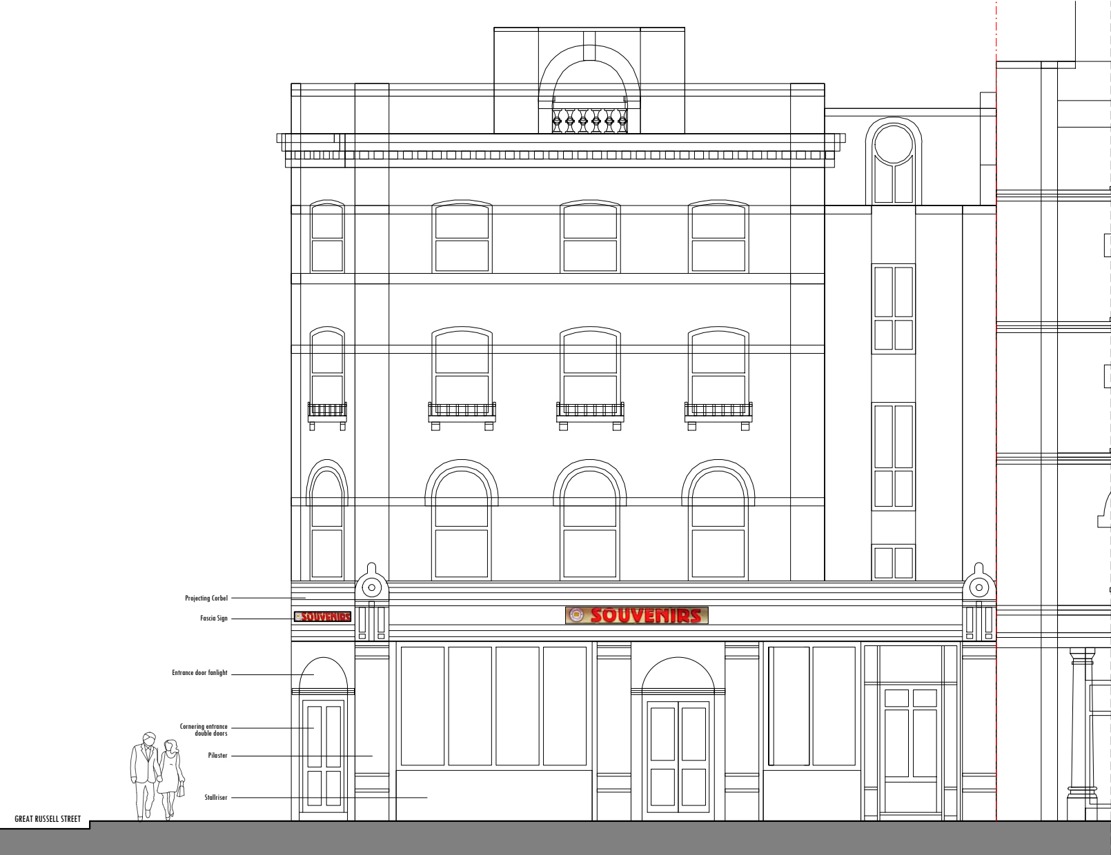
PRE-EXISTING FRONT ELEVATION - BLOOMSBURY STREET Scale:1/100
