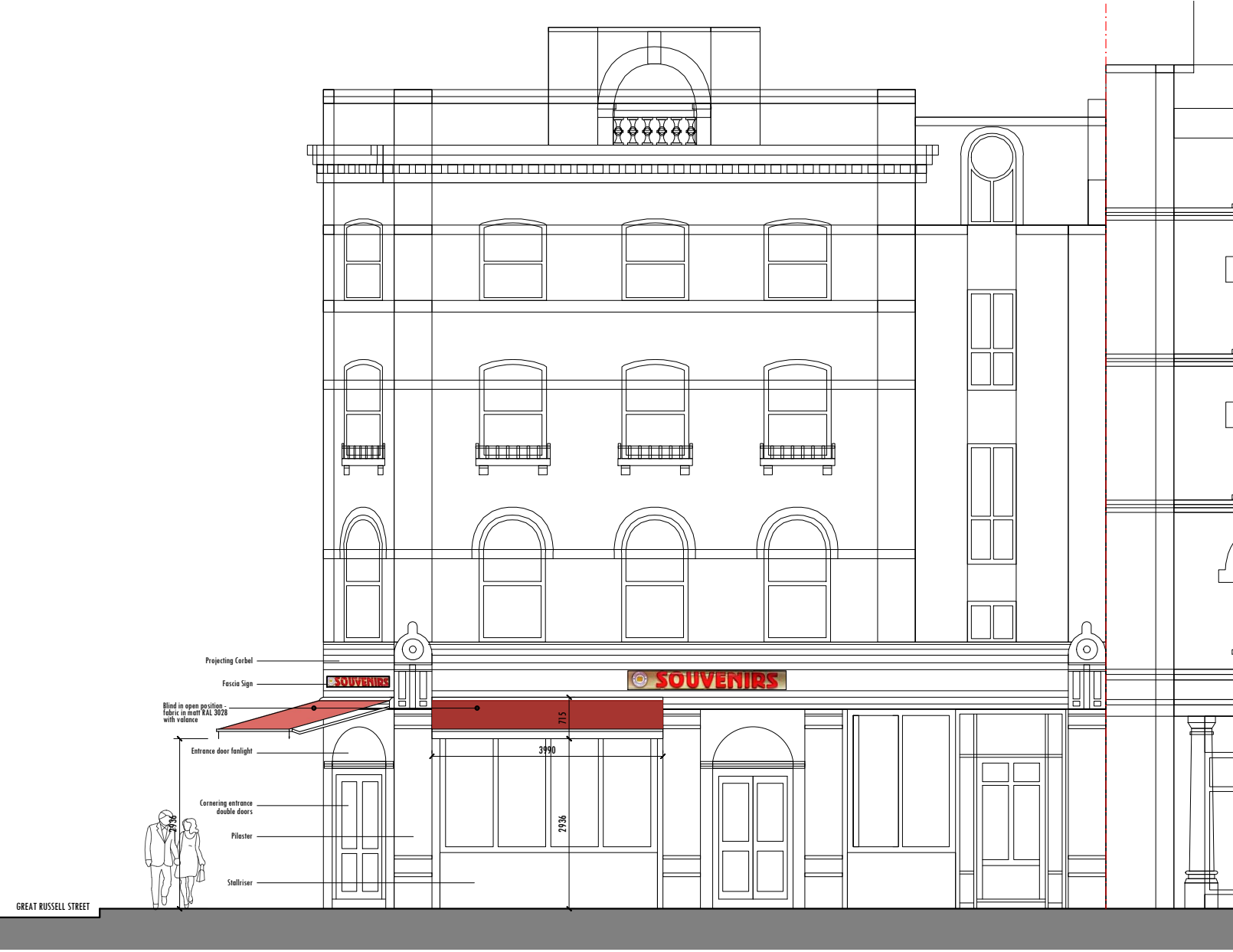
EXISTING FRONT ELEVATION - BLOOMSBURY STREET (CANOPY IN OPEN POSITION) Scale:1/100
