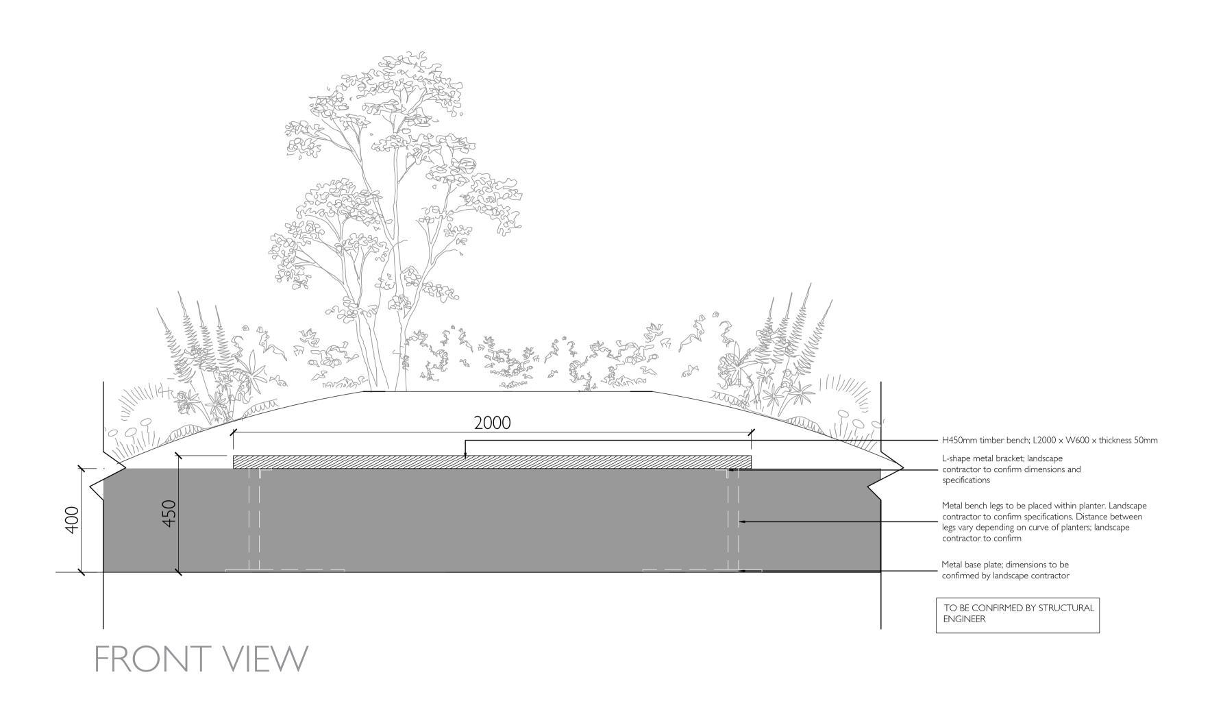
Typical Planter Bench Detail Front View @ 1:10 scale
