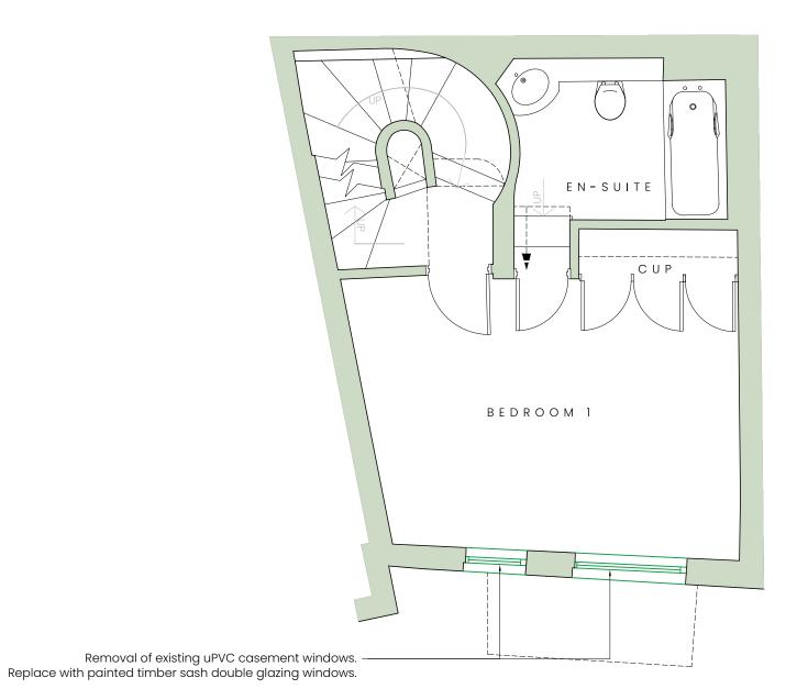
Any given dimensions on Architectural drawings require verification on site prior to any works progressing.
