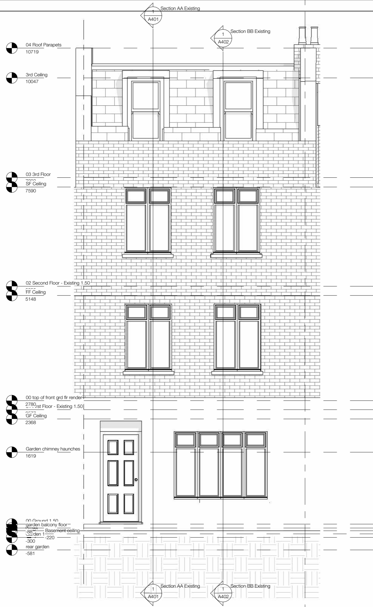
1 Front Elevation - Existing 1 : 50
