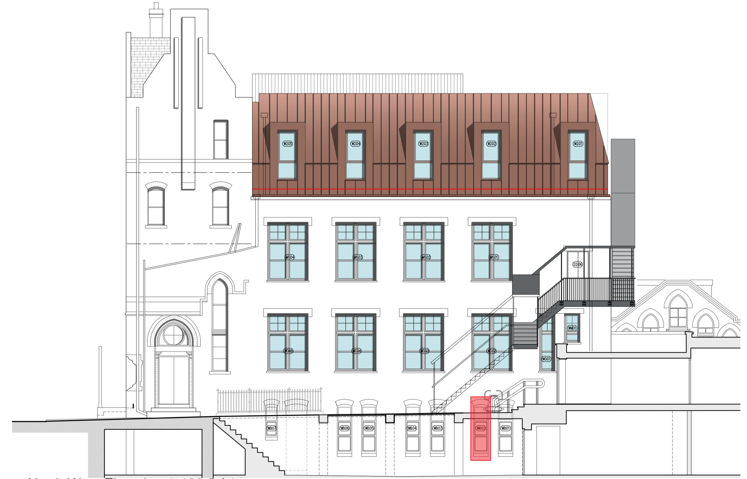
North West Elevation 1:100@A1
