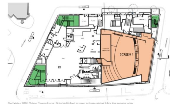
The Existing 2001 Odeon Cinema layout. Stairs highlighted in green indicate original fabric that remains today.
