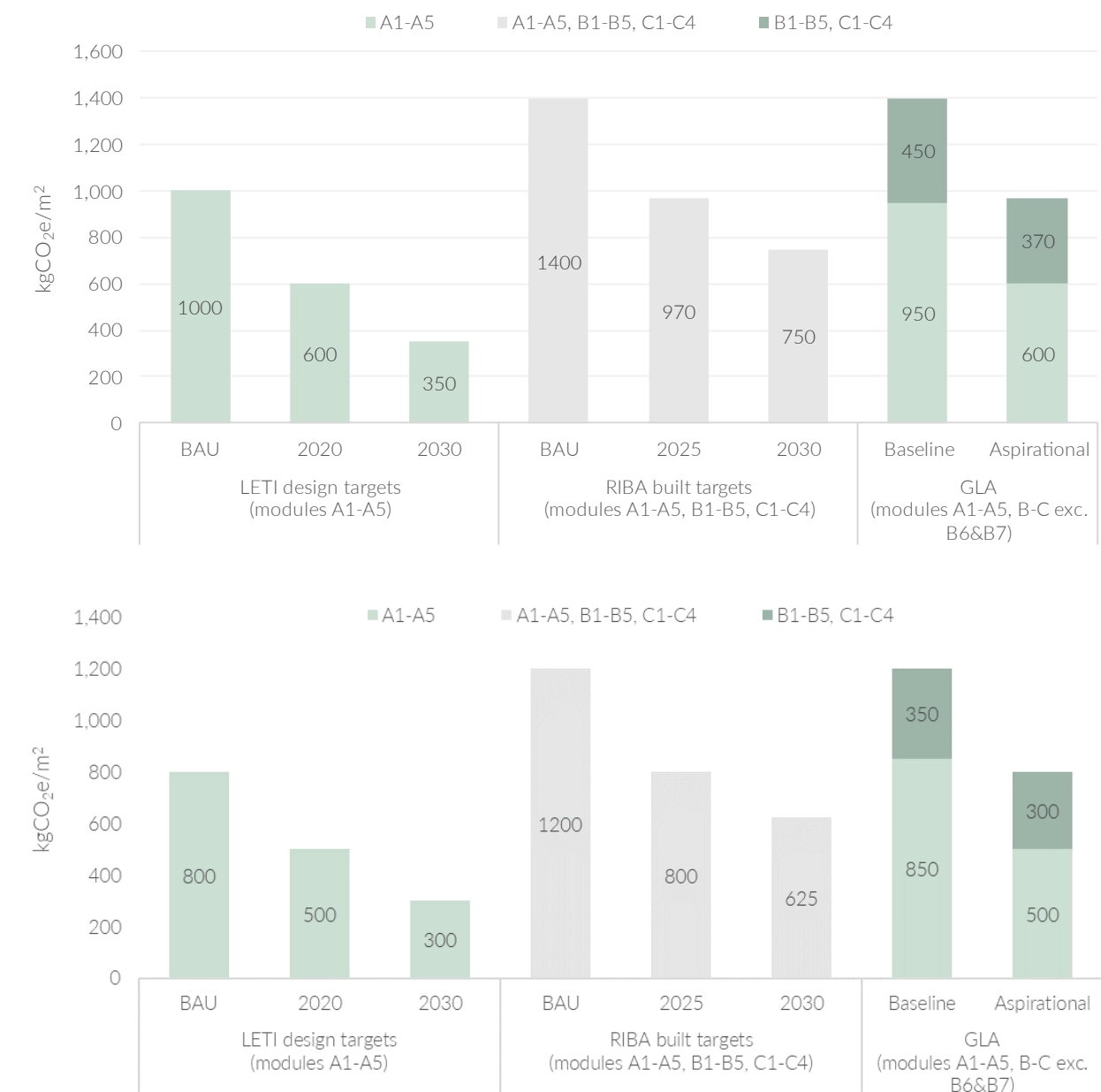
Figure 5: Embodied carbon targets for offices (top) and residential (bottom) from LETI and RIBA (Source: RIBA Climate Challenge 2020 v2, LETI embodied carbon primer).
