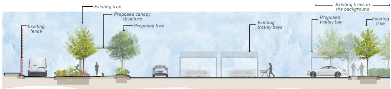
3.7m 4m 3.3m 1.4m 26.5m 3.3m London Underground Access road Planting bed Footpath Planting bed Car park Footpath with existing tree Section A-A' (Proposed)
