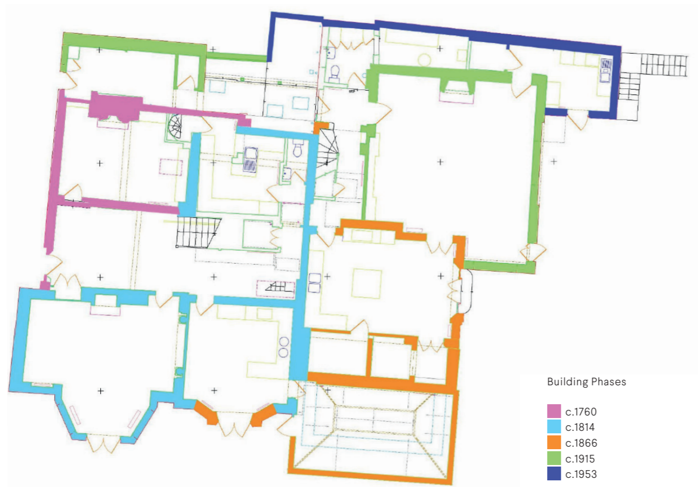
Diagram showing estimated historical building phases of 88 and 90 Frognal Credit: The Townscape Consultancy
