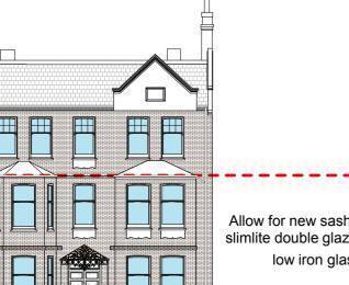
Allow for new sash windows like for like slimlite double glazing (4mm/4mm/4mm) low iron glass, argon filled
