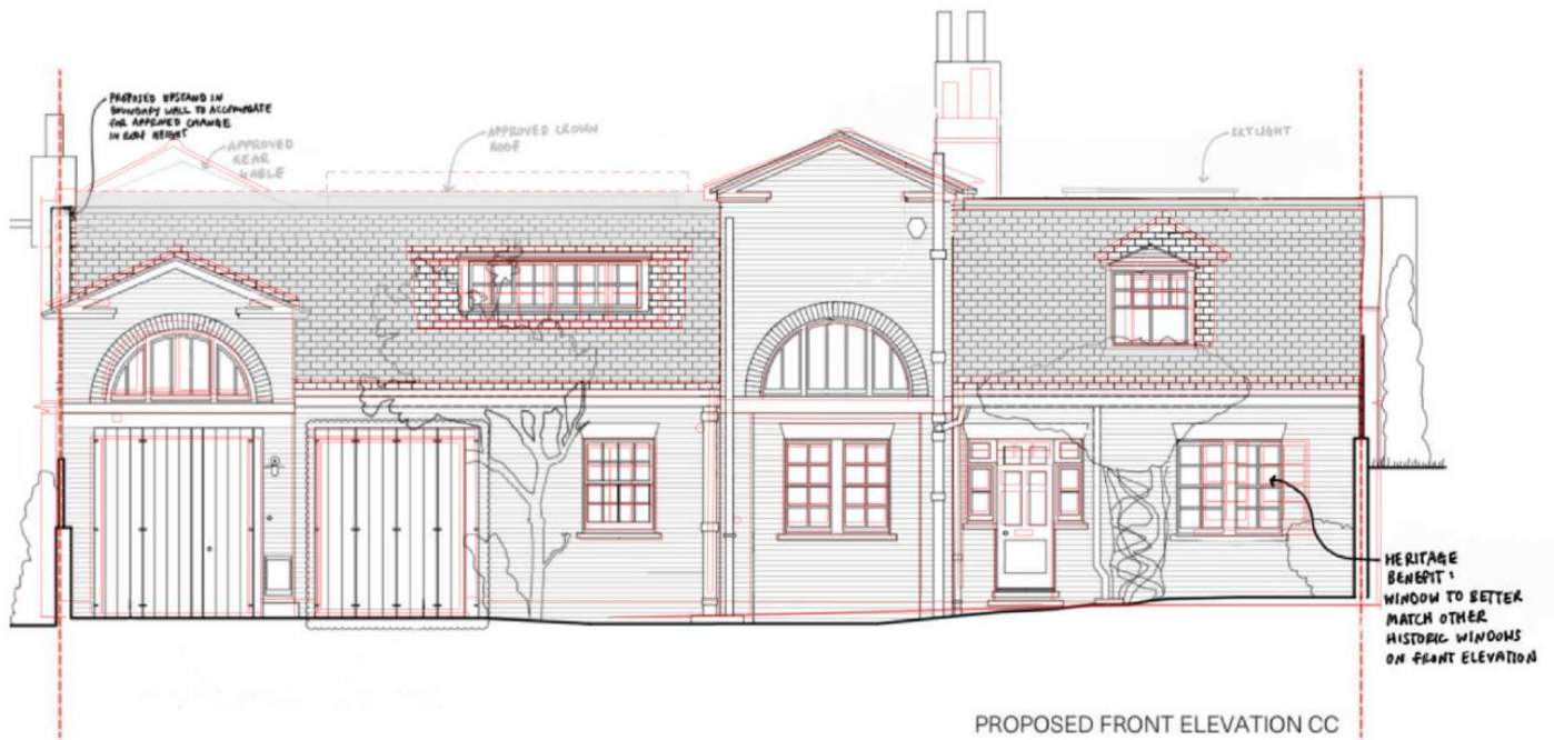
Figure 23. As built front elevation showing increase in height to the front elevation.
