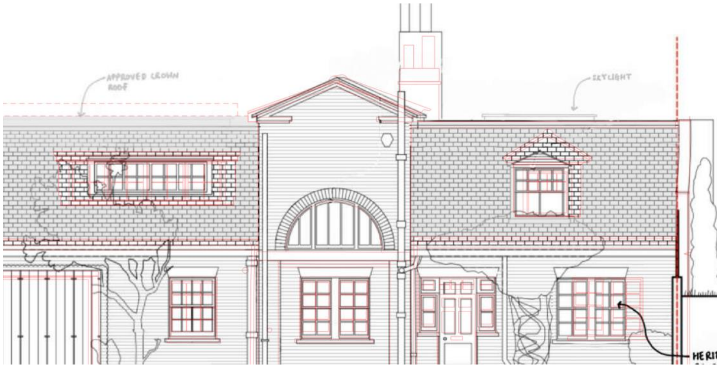
Figure 26. As built front elevation showing the as built front dormer windows in red.
