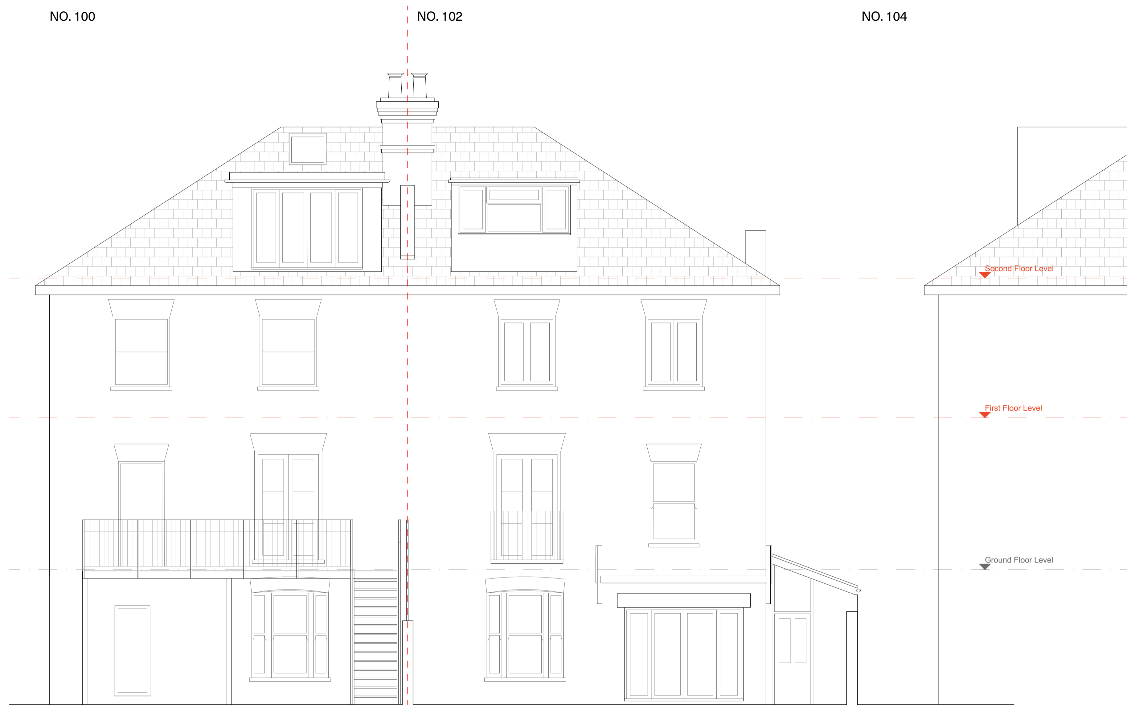
03. Existing Rear Elevation
