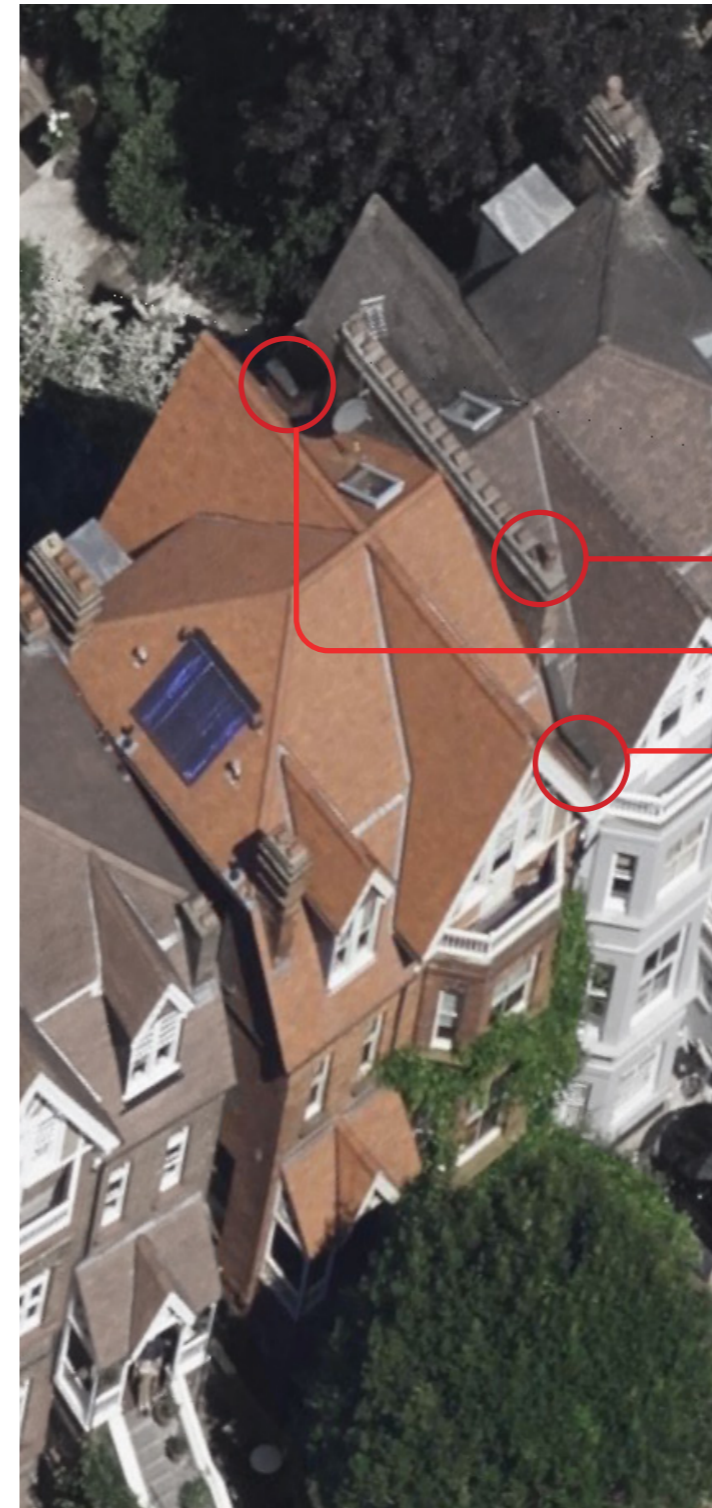
Detail of blocked gutter to the rear of the property, this requires clearance.
